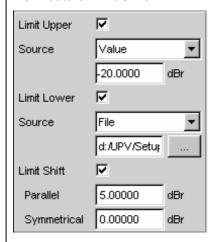
Limit lines defined by value or file can be shifted in parallel or symmetrically along the Y-Axis. This can be used to adjust the desired tolerance scheme loaded from limit files.
