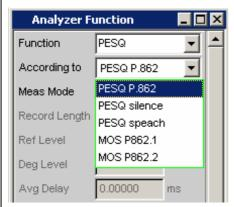
The Numeric Display shows the MOS value. The average delay is displayed in the analyzer function panel. A new display panel PESQ Graph is available showing MOS and delay versus time.
